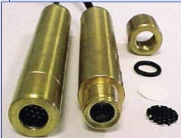
Figure 1: Hydrocarbon sensors and exploded view of sensor head
