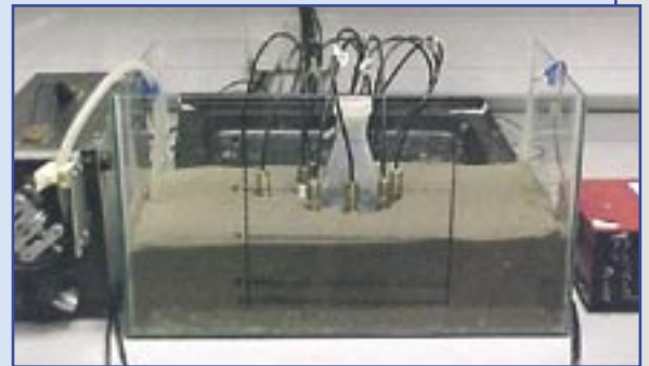
Figure 3: Laboratory trials of fuel leak sensors
