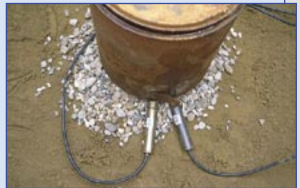
Figure 4: Positioning of sensors and leaking UST tank in lysimeter field trials
