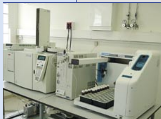
Figure 2: Fully automated P&T-GC/MS analytical system: SOLATEk 72 Multi-Matrix Vial Autosampler coupled to a Purge and Trap Concentrator Tekmar 3100 (both Tekmar-Dohrmann, USA) and a Trace GC coupled to a Voyager MS (ThermoQuest Finnigan, USA).
