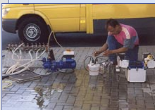
Figure 3: Sampling at multilevel well on a BTEX contaminated site in Düsseldorf, July 2003.
